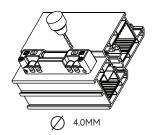
4 Lift the hinge clear, fit the hinge body and either pre-drill or fix with self drilling screws
