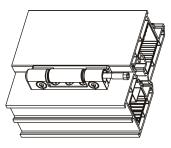
Lateral and vertical adjustment are pre-set. The hinge pin should be set so that the alignment mark points towards the sash 8 Fit cover caps if required. Top cap must be fitted as it locks the hinge pin in place
