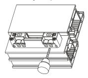
2 Lift sash clear and fit the flag to the sash
