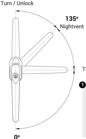
Release button using the key. Handle is now free to move past 90° for Turn or Nightvent mode.
