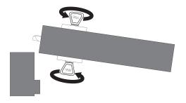
With door open, operate cylinder from both sides to ensure smooth operation. **NEVER** use the key as a handle to open or close the door. Repeat process with door closed ensuring deadbolt engages correctly with the keep. Adjust if necessary.
