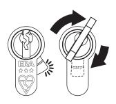
To remove your existing cylinder, open the door. With the key inserted into the cylinder, rotate slightly to align cam with cylinder body to allow installation.
