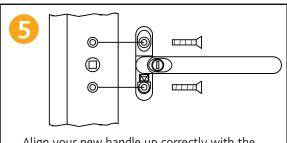
Align your new handle up correctly with the new existing holes in your window and fit the handle using the correct size screws which should be provided within the packaging. Once securely fitted, turn the handle into the locked position and back again into the unlocked position to ensure the correct operation.
