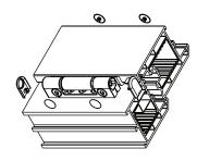
3 Clip jig under flag barrel. Drill the two holes for the hinge pins
