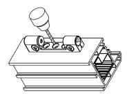
Lateral and vertical adjustment are pre-set. The hinge pin should be set so that the alignment mark points towards the sash
