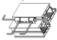
2 Lower the sash into the frame, ensure correct placement, clamp if necessary
