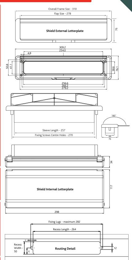
All dimensions are in mm. Fab&Fix reserves the right to change specification without notice. It is the responsibility of the door manufacturer to ensure that the finished product meets any required safety and performance specification.
